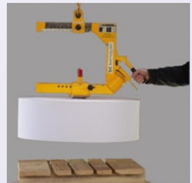
3. Lifting, gripping acts automatically
