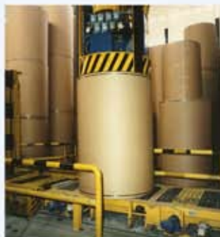
3. At slack rope suction gripping happens automatically
