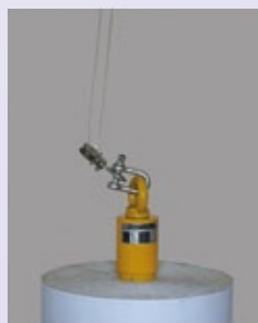
3. At slack rope, automatic switch to gripping
